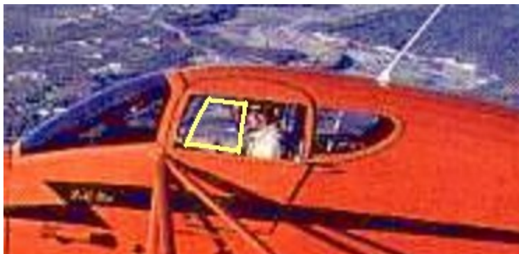
Fig.26 The CallAir pilot position in relation to the opening side window pane (outlined in yellow) 239
