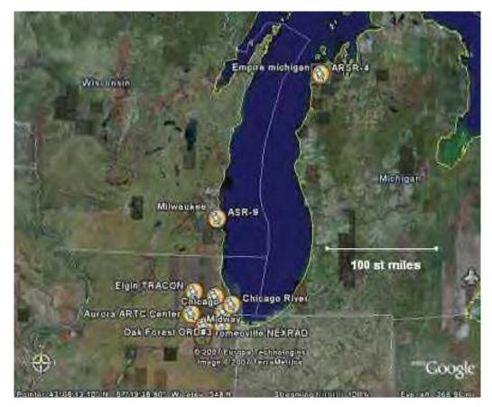
Fig.4. Radar locations around Lake Michigan. Showing the ARSR-4 at Empire, Michigan, and ASR-9 at Milwaukee. The maximum range of the latter falls a few miles short of the area of the incident at Chicago O'Hare.
